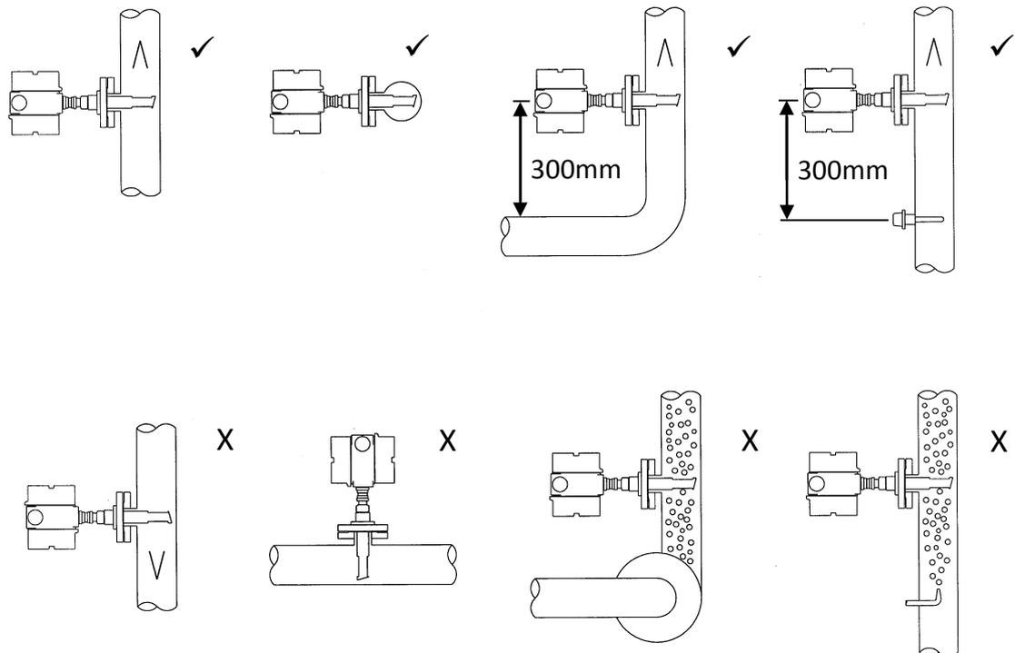
1. Liquid flowing vertically upwards is preferred to a horizontal pipe or vertical downward pipe as it is more likely to always remain full of liquid. **The sensor must be fully submerged otherwise there will be no echo from the reflector.**
